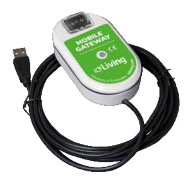
The Mobile Gateway receives data from ioLiving measurement devices and transfers it to the ioLiving cloud service via mobile network.
