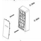
Step 1: Mount the AURA unit on the wall with 2, ISO #6, 25mmL, CSK (+) screws as shown below
