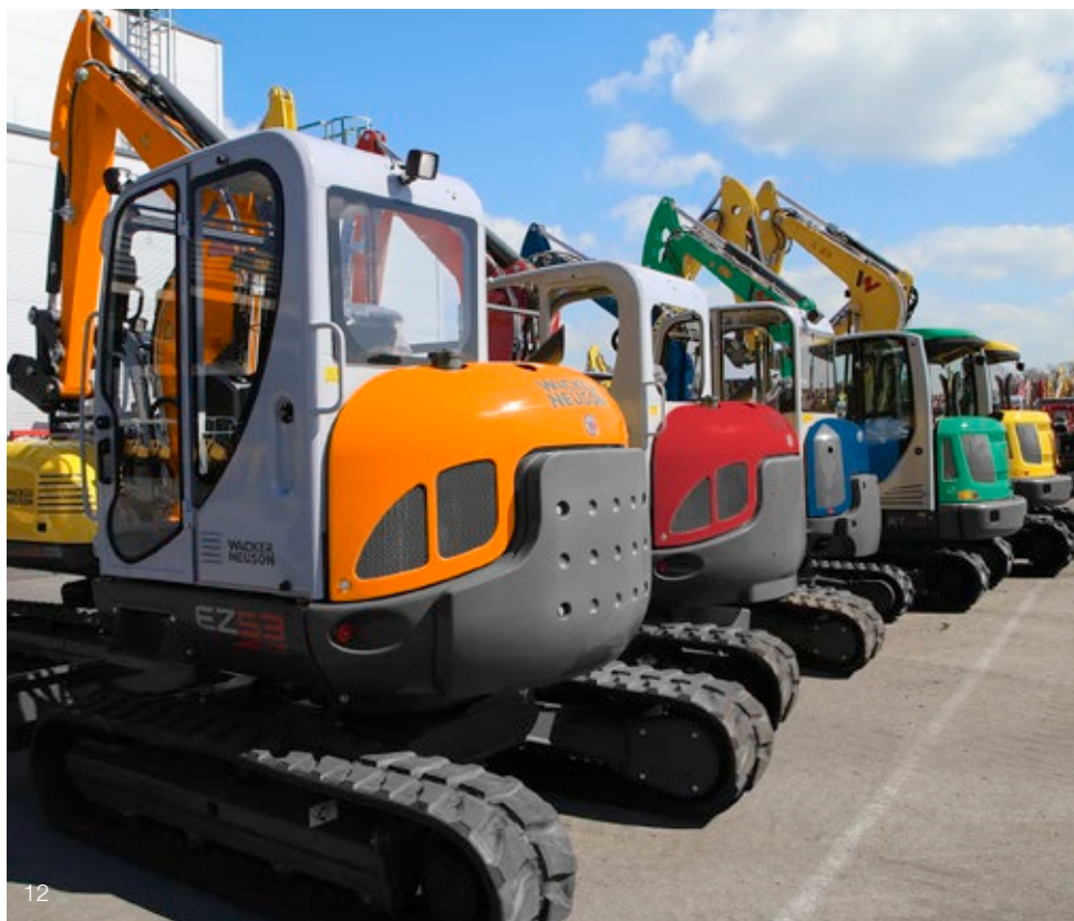
Attachment carrier with many application areas thanks to up to 5 additional control circuits.
