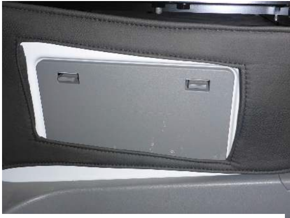
The heat exchanger access panel on the outboard side of the passenger seat pedestal
