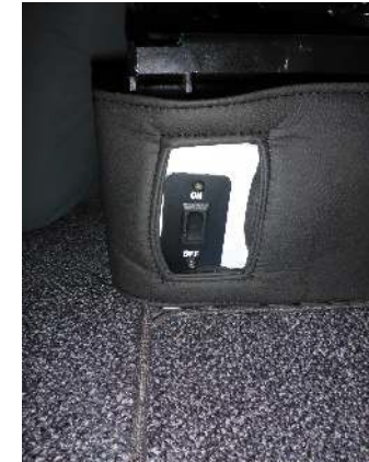
The switch is located on the inboard side of the passenger seat pedestal
