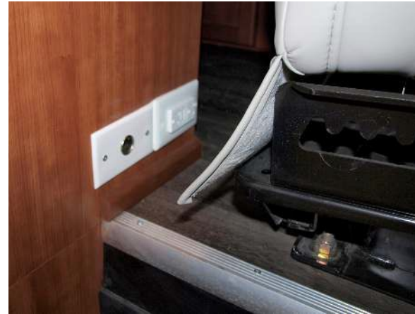
GFCI plug behind rear captain's seat
