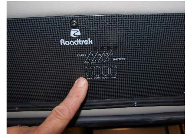
Tank and battery level indicators
