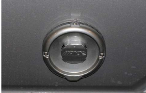
Vent for Alde unit on driver's side exterior
