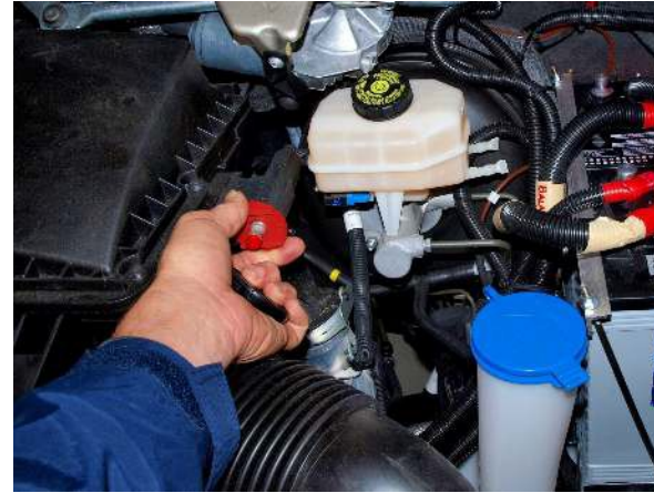
Positive jumper point, on driver's side of the engine. Red disc is pushed back to expose the contact
