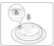
Install the burner head so that the electrode passes through the opening for the electrode. Make sure the burner head lies flat on the stove top.
