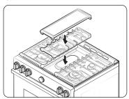
The griddle can be used only with the center burner on the center grate. Use caution when putting the griddle on the center grate.
