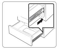
**4.** Put the drawer in the roller guides on either side, and then snap the clips into place.
