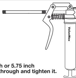
Select the 4.25 inch or 5.75 inch extension, thread through and tighten it.
