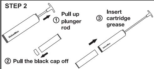
**CAUTION:** Make sure pull up plunger rod to the end, the plunger rod will be locked.
