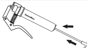
Grasp T-handle and pulling back slightly then keep pressing rod lock to release. Push on plunger rod T-handle to force plunger into cartridge.
