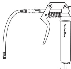
Attach the flexible hose to the nozzle threads.
