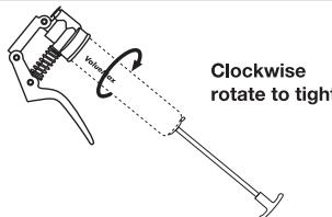
**CAUTION:** Peel off the foil cover before tightening. Before tightening the grease gun head, never press the lock, otherwise grease may spray!
