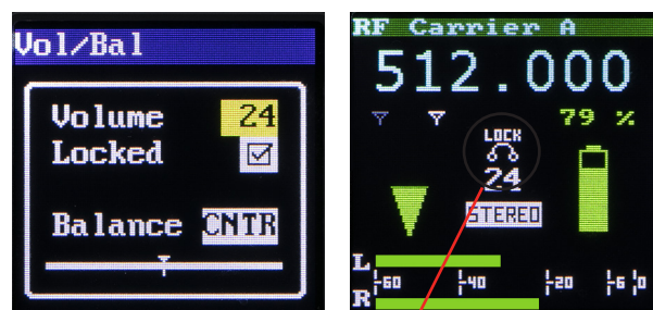
Volume locked display on main screen
