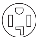
4-wire receptacle (14-30R)
