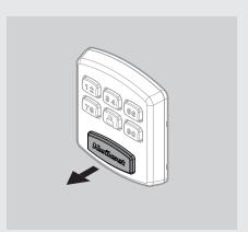
Hold the battery to the terminals. You will hear beeping to signal you can open door.
