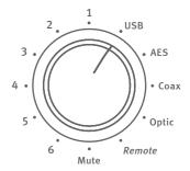
Select one of the six analog inputs 1 - 6. Select one digital input USB, AES, Coax or Optic.
