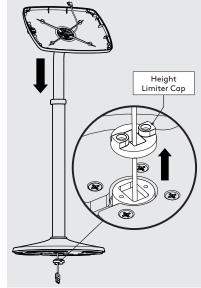
Locate & secure the Case onto the Elevate Pole as shown. Tighten by hand.
