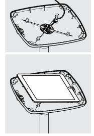
Install the Tablet into the 11 Case & connect to Power Cable.
