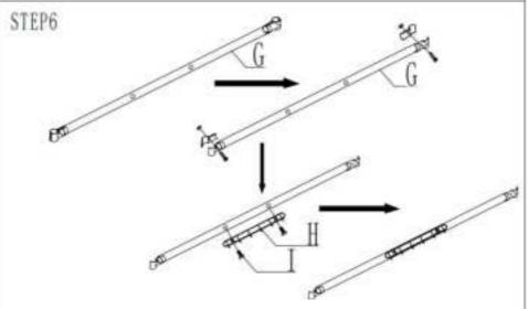
Loosen the screws on the fixing pieces at both ends of accessory G, remove the half as shown in the figure, and then fix accessory H to the G tube by means of the screws.
