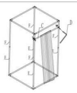
According to the user's high-level requirements, after assembling step 4 onto the appropriate position of the F tube, tighten the screws.
