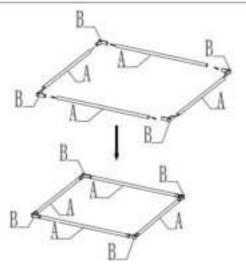
Don't tighten the screws of Accessories A and B too much. Just tighten them to 60% of the full capacity. Assemble two sets.
