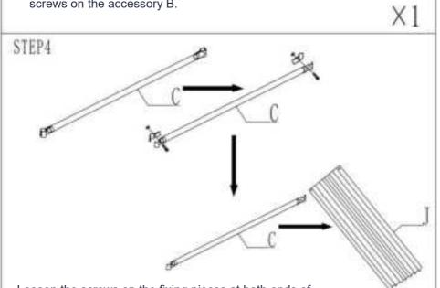
Loosen the screws on the fixing pieces at both ends of accessory C, remove the half as shown in the figure, and then insert the curtain J into the C rod.
