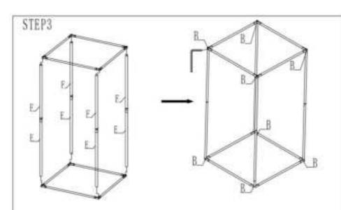
Assemble Step 1 and Step 2 together, and then tighten the screws on the accessory B.
