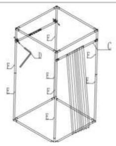
According to the user's requirements, after assembling Step 6 in the appropriate position of the F tube, tighten the screws.
