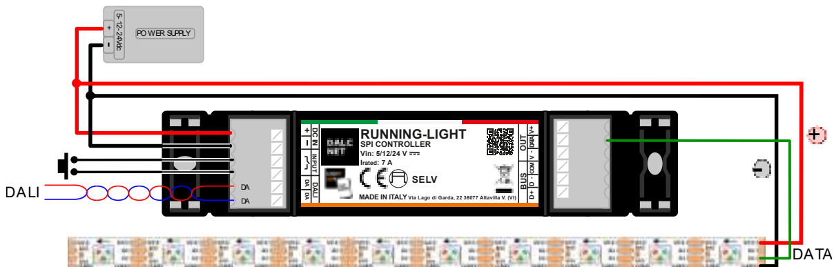
Figure 3: Connection diagram for Digital LED loads (> 7A)
