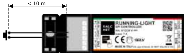
Figure 4: Local Command wiring diagram for Short Distances
