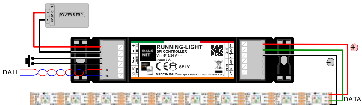
Figure 2: Connection diagram for Digital LED loads
