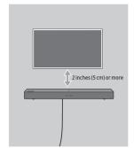
For Installation on Concrete Walls (not supplied)
