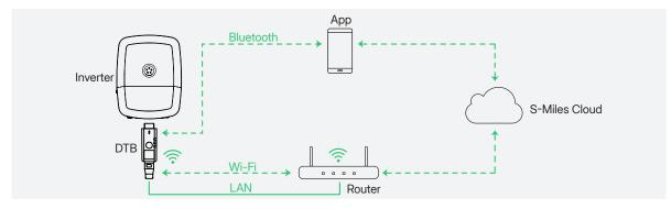
\* DTB Interface: Connect and communicate with the inverter. Inverter Interface: Connect and communicate with the DTB. DTS User Manual Product Introduction
