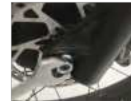
5. Install the front fork and tighten the screws and nuts
