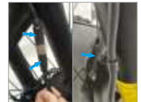
6. · Connect the motor wire (note that the arrows on both ends of the connector correspond) · Install the motor wire holder
