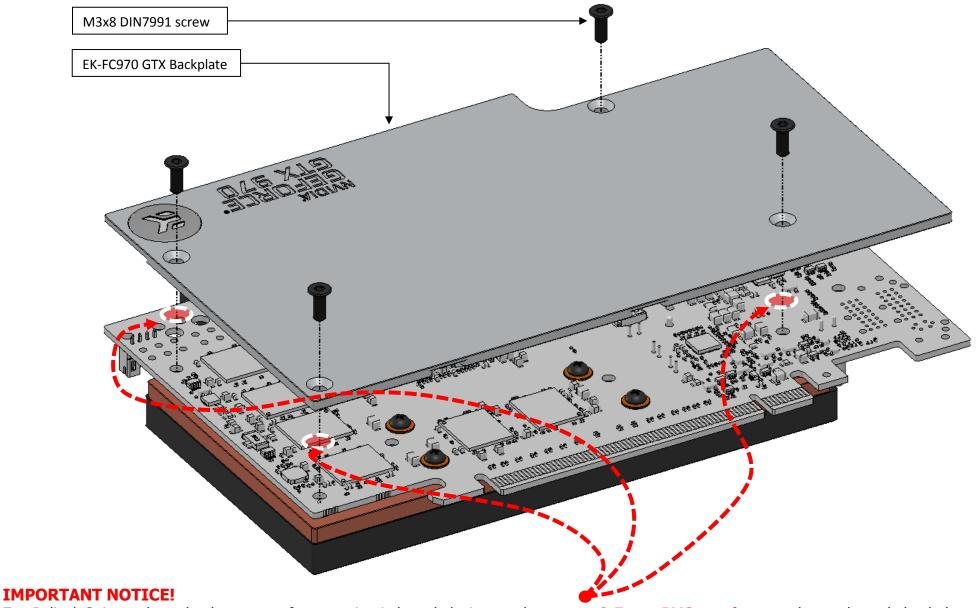
For Palit / Gainward- and other non-reference circuit board design – please use <u>0.5mm PVC washers</u> underneath each backplate standoff to prevent backplate collision with tantalum capacitors or other circuit board components. When using 0.5mm washers it is **mandatory to use 1mm thermal pad** on memory IC (if present) instead of 0.5mm (as shown in STEP 3).
