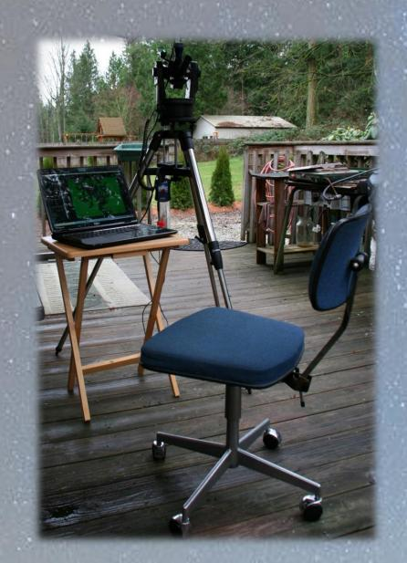
The photo on the left shows a Meade ETX 90 that has been outfitted with a Meade LPI-G Advanced Color camera. (Lunar Planetary Imager and Guilder) The camera is connected to a Laptop Computer which is running Meade's "Sky Capture" software. There is many more similar software packages on the market that might be superior and the job of these software packages is to get what the telescope is currently viewing in real time onto the computer screen.
