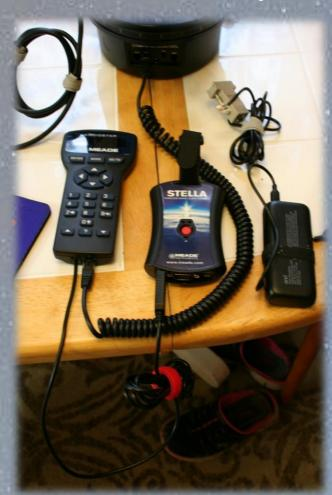
The photo on the left shows some details of what the connection pattern between the telescope, AudioStar Handset and the Stella WiFi adapter would look like. The AudioStar Handset is connected to the telescope base as normal. There is also a secondary connection using the Meade #505 Cable Set going from the handset to the Stella.
