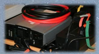
Another option is a large DC Power Cell hooked up to an Inverter that converts DC power to AC power. You have to figure out how many total watts in power your system will need.
