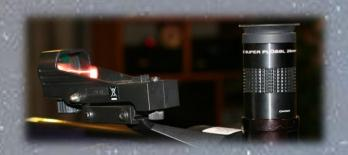
Some models of the ETX, depending on date of manufacture, have different Finder Scopes. Some have an electronic red dot and others might have a low power scope with crosshairs, mounted to the main telescope body.
