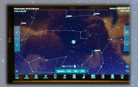
Stella sets up a WiFi network which can be connected to a handheld device such as a computer tablet. A special StellaAccess application has to be downloaded and the application is available on both Apple's iOS and Android platforms. Once the app is downloaded and opened, one has to set it up, meaning telling the app such things as what telescope is actually going to be used.
