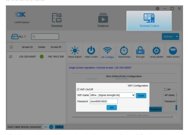
After about 3 minutes, the control card will automatically search for the WiFi hotspot connected to the configuration, and the "internet" light on the control card will flash uniformly and slowly, indicating that it has connected to the cloud platform. At this time, you can log in to the cloud platform www.m2mled.net to send the program.
