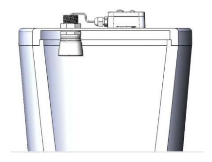
5. If the top of the water tank cannot be opened, the hole made on the top of the water tank is recommended to be 45mm diameter. It is recommended to add a gasket (size: 32.4\*57.4\*3mm) between the hole and the sensor.
