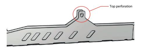
Insert the original screw into the top hole and one 1/4" x 2 1/2" screws in the perforations of the rear suspension thightening with double washers and one nut of 1/4".
