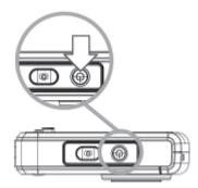
Press the **U** POWER button to turn on the camera.
