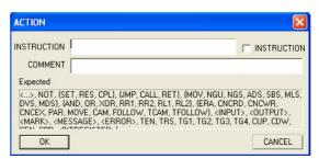
The instruction must be written in mnemonic language. Placing the cursor on action\_contact and using the "Parallel" softkey, it is possible to add other action\_contact in parallel.
