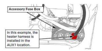
5. Use the diagram on the underside of the fuse cover to **locate and remove** the 10A fuse for the connector location that the heater's power lead is connected to.
