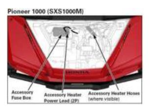
3. Remove the fuse cover from the Accessory Fuse Box by depressing the two lock tabs.
