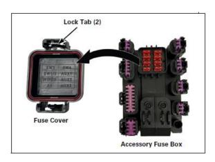
4. Locate the Accessory Heater harness and power lead, and then identify which fuse box connector location the power lead 2-pin connector is installed in.
