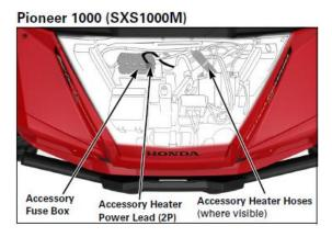
3. Remove the fuse cover from the Accessory Fuse Box by depressing the two lock tabs.
