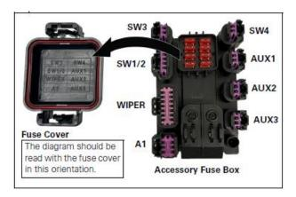
6. Store the removed 10A fuse in the vehicle's main fuse box in the open spare fuse holder.
