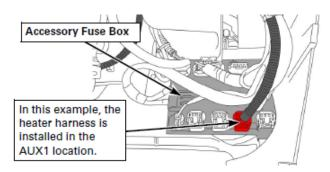
5. Use the diagram on the underside of the fuse cover to **locate and remove** the 10A fuse for the connector location that the heater's power lead is connected to.
