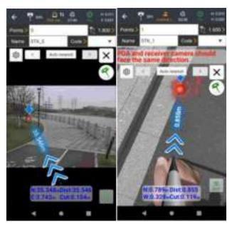
(4) In the video, the target stakeout point appears as a red dot. When the virtual pole tip touches the dot, you've reached the point. Tap the stakeout icon and the point is automatically saved.
