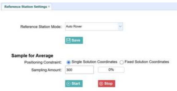
Use this screen to configure settings such as the station coordinates and the broadcast station identifiers. You must enter accurate information in these fields, as this data affects the accuracy of logged data files and broadcast correction data significantly:
