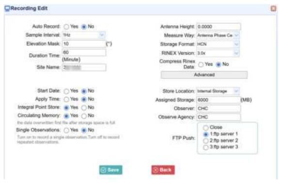
In this screen, you can configure all the data logging parameters, and determine whether the recording files will be affected by the FTP Push. The parameters are mainly as follows:
