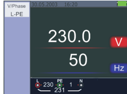
Figure 5.2.7.2 Screen while measuring Voltage and Frequency
