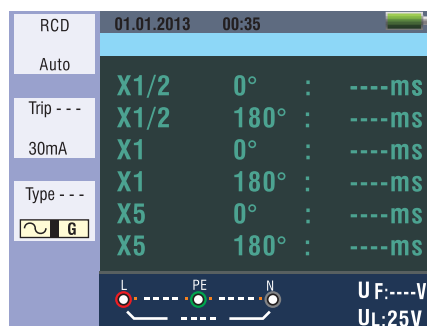
Figure 5.2.5.1.1 RCD Auto Function Screen
