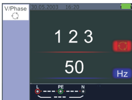
Figure 5.2.8.3 Phase Sequence screen -when connected in clockwise direction.
