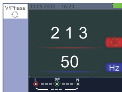
Figure 5.2.8.4 Phase Sequence – When connected in counter-clockwise manner
