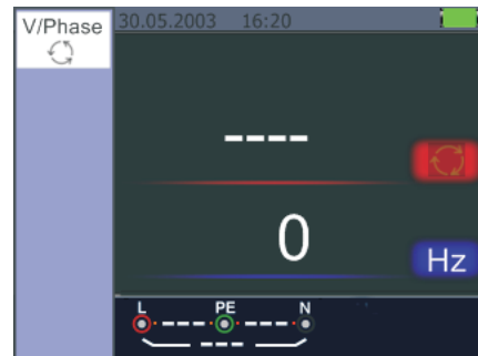
Figure 5.2.8.1 Initial screen of the Phase Sequence Measurement
