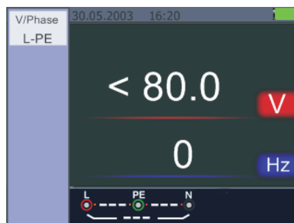
Figure 5.2.7.1 Standby screen for the Voltage and Frequency
