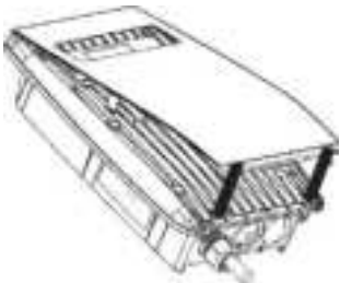
Install torque 3-4 lb-in (0.3-0.5 N-m)
