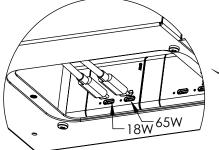
REPLACE THE ACCESS HATCH AND PLUG IN CONNECTOR TO POWER THE UNIT
