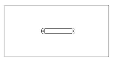
PRECISION MACHINE CUTOUT INTO DESK OR JOINERY AS PER THE SIZE/TOLERENCE LISTED ON THE TECHNICAL DRAWING OF THE MODEL SELECTED
