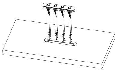
INSTALLING THE USB UNIT INTO THE CUTOUT-INSTALL USB CABLES INTO THE KEYSTONE JACKS (NOTING THE CORRECT ALIGNMENT OF THE CONNECTIONS)
