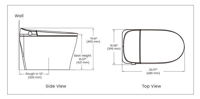
To ensure proper installation, the distance between the water supply valve and the centerline of the toilet should be greater than half the width of the toilet bottom. The water supply valve should be about 8 inches away from the toilet centerline. For larger valves, a greater distance may be necessary to ensure proper clearance. For easy installation and maintenance, a range of 9 to 11 inches is recommended.
