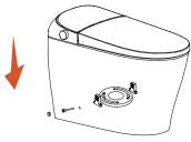
Insert the screw through the fixing sleeve, then through the holes on both sides of the ceramic toilet and into the mounting blocks on the ground. Tighten them securely using a screwdriver.
