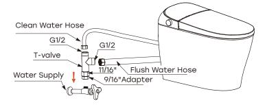
Note: If your water valve is 9/16", you could directly connect the T-valve; If your water valve is 11/16", please screw off the adapter, then connect it.
