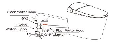
Connect the smaller clean water hose to the T-valve and tighten it.
