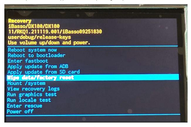
13. Use volume wheel to select WIPE Data/Factory RESET and select Factory Data Reset
