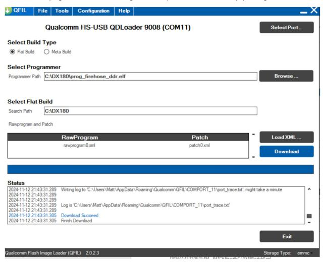
You should see FLASH DOWNLOADED and at this point the DAP now has the FW installed. You can unplug the DAP and power on now. Before we wipe data several times we will need to get 2 files off the DAP so leave QFIL open.
