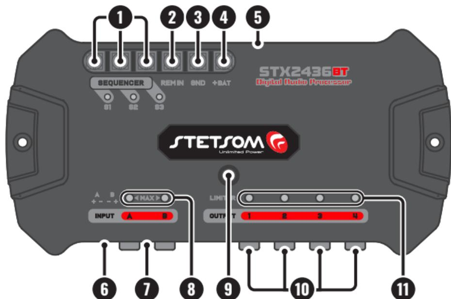
**1. SEQUENCER:** This feature allows sequenced startup of other products through your remote connection (REM). Make the connection using a minimum **18 AWG** cable. Each connection can be configured, enabled or disabled by the application or SMC control.
