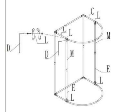
First, separate the accessory L as shown in the figure. Then install accessory L to the position marked on the C tube, and do not tighten the screws yet.
