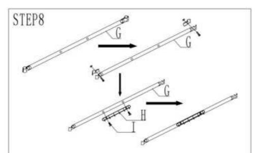
Loosen the screws on the fixing piece at both ends of accessory G, and remove half of it as shown in the figure.
