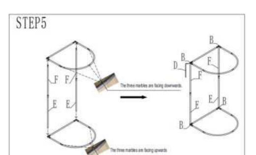
As shown in the figure, after installation, tighten all the screws.
