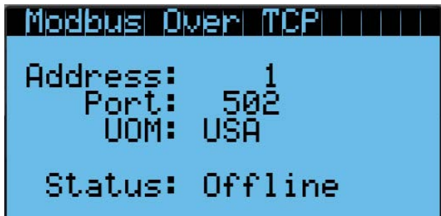
FIGURE 25 Modbus TCP Setup
