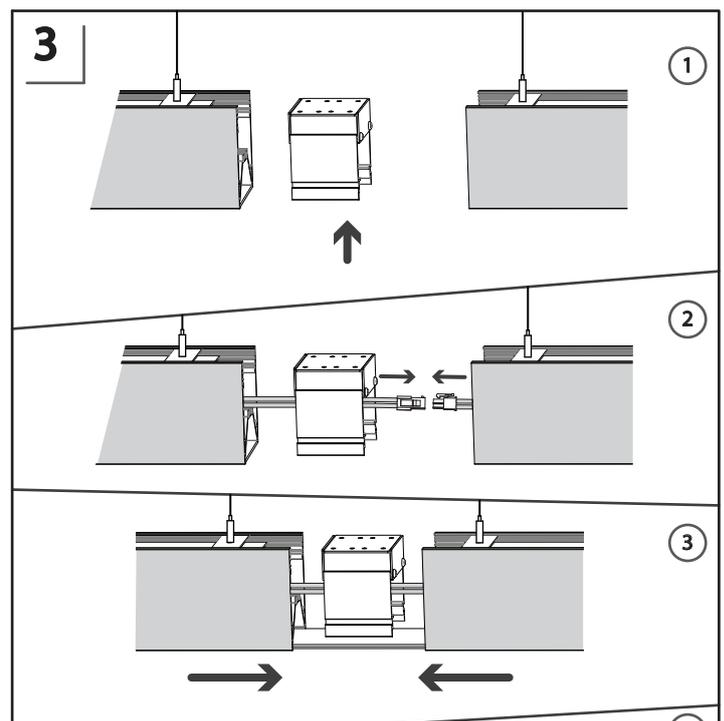
Connection bracket is not designed to handle the excessive load, caused by incorrect luminaire installation!
