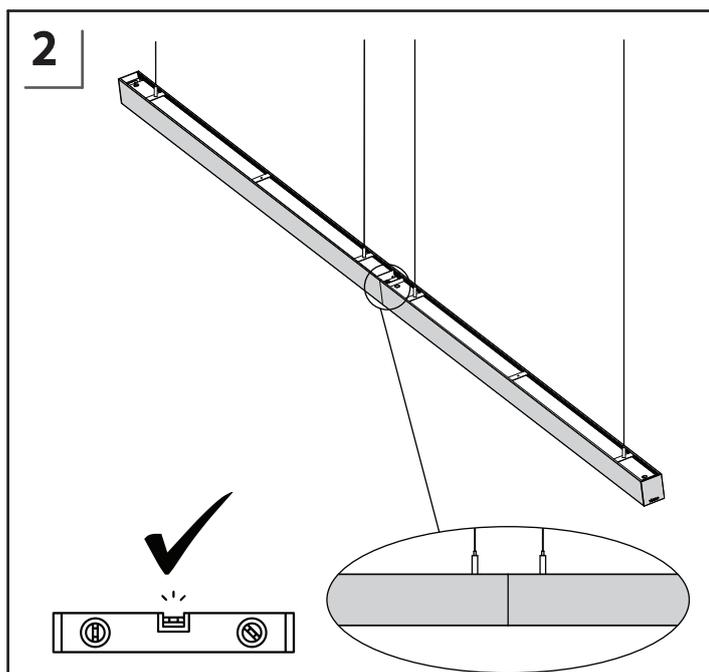
Modules should be parallel, aligned, without a gap in between before installing a connection bracket in order not to create excessive load!
