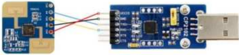
Figure 4-1 Connection between HLK-LD2420 hardware and USB serial port adapter board
