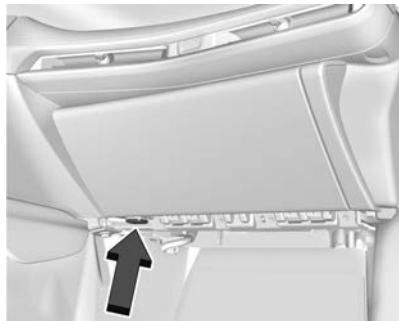
Interior Power Outlet
