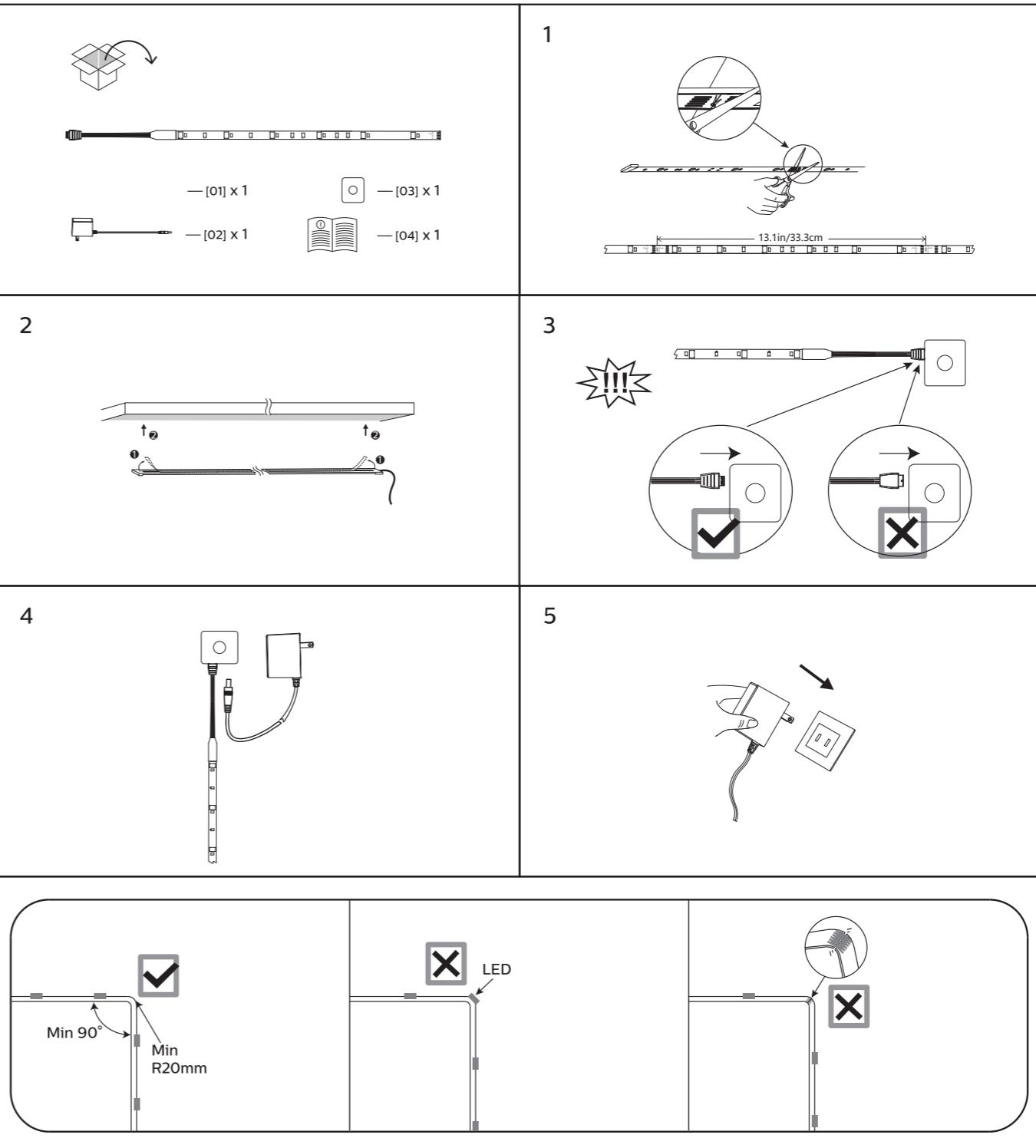
Only use the control box provided in this kit to control this light strip. This lamp will not operate properly when connected to a standard (incandescent) dimmer or dimming control device.
