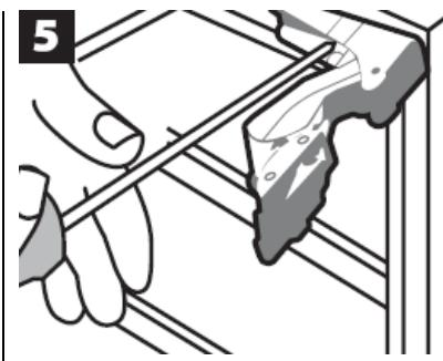
With the hinge open undo the screws of the top hinge.
