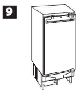
Check that the door is adjusted properly. Check that the door seals close properly. Finally tighten the screws.
