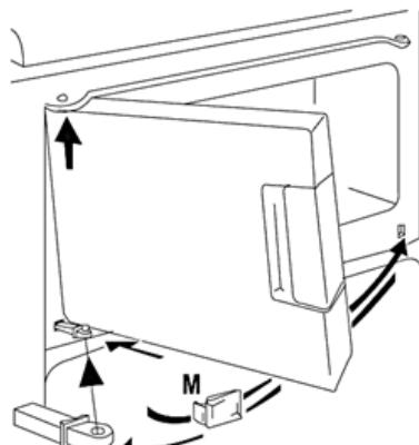
Slightly open the freezer compartment door. Using a small screwdriver, press the spring in the opening of the lower door bearing slightly upwards and take out the door bearing and the door. Install the cover cap (M) on the opposite side. Turn the
