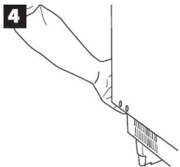
Support the bottom of the door. Be careful with the hinges. Remove the door.
