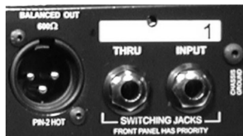
Fig. 2 A convenient chassis ground is provided to allow alternate ground schemes
