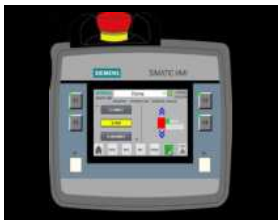
Figure 28: HMI Displays Device in TEST (amber indication) Position
