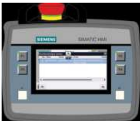
Figure 23: HMI Shown with Alarm Log
