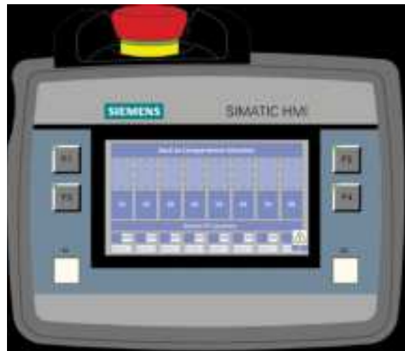
Figure 33: HMI Display showing section selection in a lower compartment
