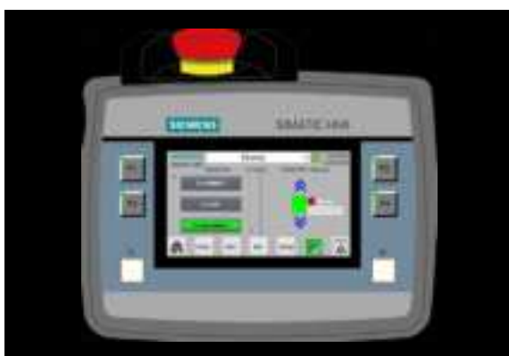
Figure 26: HMI Displays Device in DISCONNECT (green indication) Position
