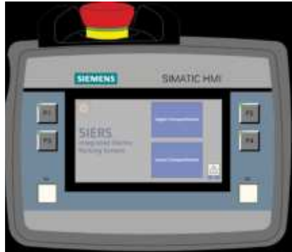
Figure 32: HMI Display showing compartment selection screen
