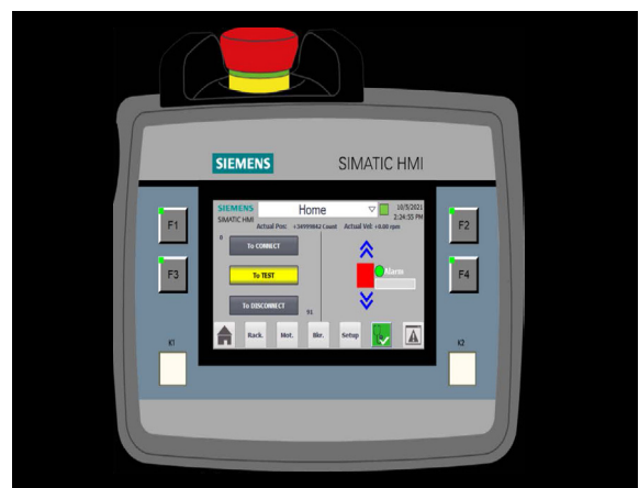
Figure 14: Displays Device in TEST (amber indication) position
