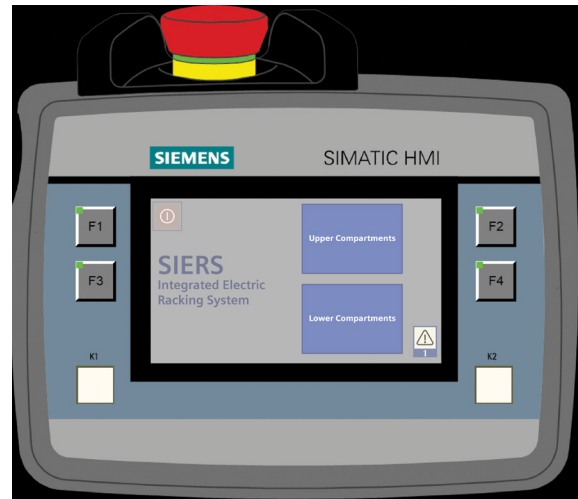
Figure 32: HMI Display showing compartment selection screen
