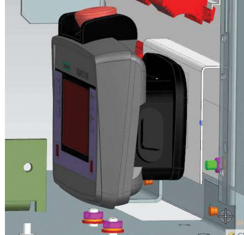
Figure 22: Portable HMI stored and mounted bracket inside low voltage compartment
