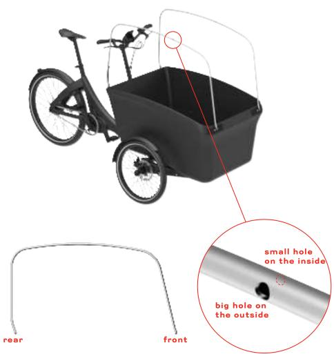
**4-** Take the 2 side frame tubes and insert them into the front and rear brackets pins. The big holes have to point to the outside.
