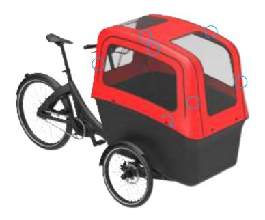
**6-** Take the 8 turn locks and mount them on the prepared positions, shown by the red circles, using 2x M3.5x13 screws on each lock.
