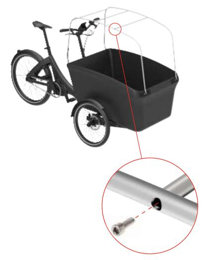
**5-** Take the 2 (2 kids hood) or 3 (4 kids hood) short straight bars and fix them to the side frame tubes with the DIN912 M4x8 screws.
