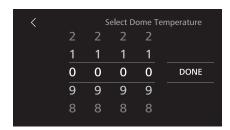
4. Adjust Deck Temperature using the scroll wheels, then select **Done**.
