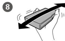
Shake the ink cartridge horizontally for 5 seconds, moving it back and forth about 10 cm 15 times.
