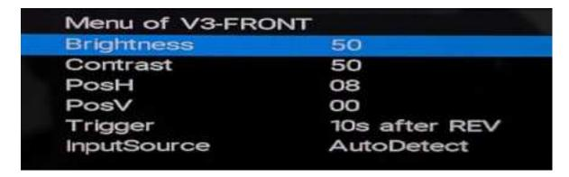
**Trigger**: select the desired time to show the <u>Front cam picture automatically after reversing</u>.
