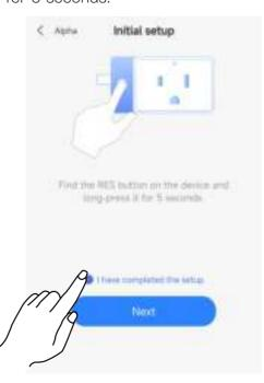
4. Set up Wi-Fi connection, it only works with 2.4G Wi-Fi network.
