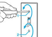
Remove the switch and pull it away from the wall.
