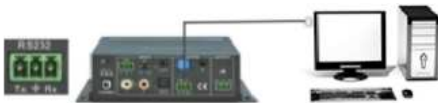
Figure 10 Connection of RS232 Port
