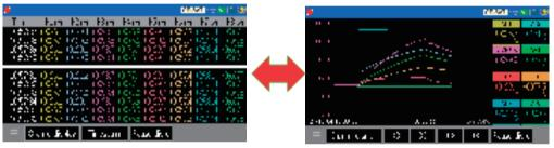
The graph indicates an elapsed time (horizontal axis) and change of measured data for each channel. On the right side of the screen (table), channel numbers and measured data are displayed. The value in the table is the latest result while measuring.
